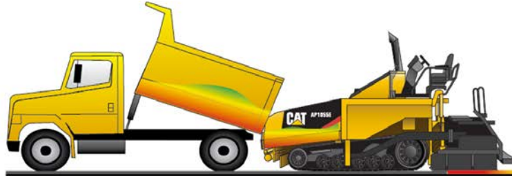
Traditional Paving Method - Particulate and thermal segregation from plant-to-paver-to-mat results in inconsistent mat temperatures and smoothness
