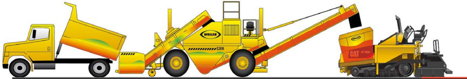
Weiler E2850 - 25-ton storage with remixing allows for non-contact, non-stop paving while reducing particulate and thermal segregation for consistent mat temperatures and smoothness
