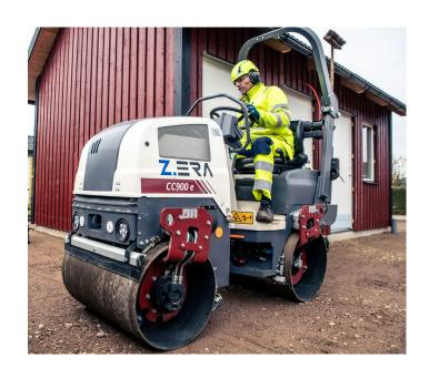
1.7 t Operating weight 9.5 kg/cm Static linear load
