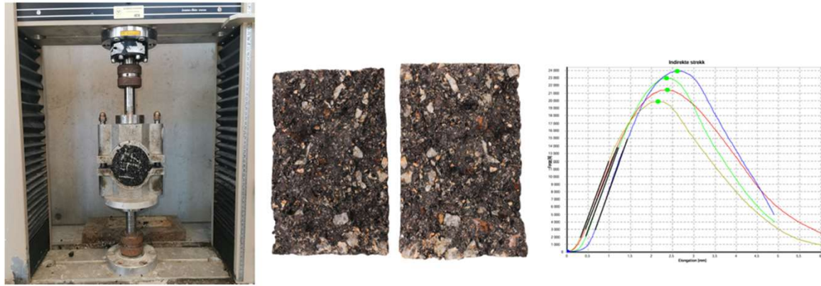
Figure 3.6: The asphalt sample in the ITS machine (left), producing two fracture surfaces (middle) and corresponding compression graph of 4 samples (right).
