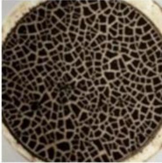
Representative asphaltene filter residues, ordered by asphaltene content
