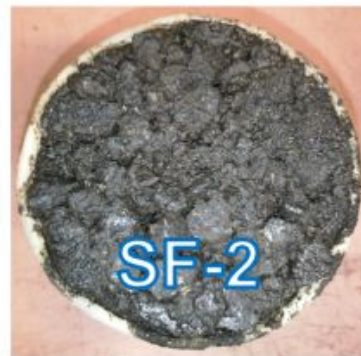
Fig. 3. RLTT samples treated with synthetic fluid according to different percentages: 0% (UGM), 1.5% (SF-1), 2.5% (SF-2) and 4.5% (SF-3), SF samples have w = 1\% .
