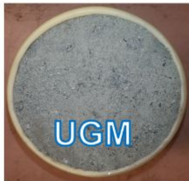
Fig. 3. RLTT samples treated with synthetic fluid according to different percentages: 0% (UGM), 1.5% (SF-1), 2.5% (SF-2) and 4.5% (SF-3), SF samples have w = 1\% .
