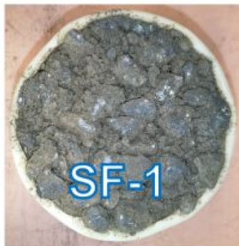
Fig. 3. RLTT samples treated with synthetic fluid according to different percentages: 0% (UGM), 1.5% (SF-1), 2.5% (SF-2) and 4.5% (SF-3), SF samples have w = 1\% .
