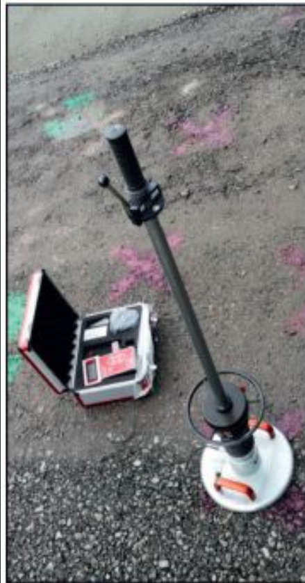
FIGURE 6: Components of the LWD and DCP used in the field test [56, 57].
